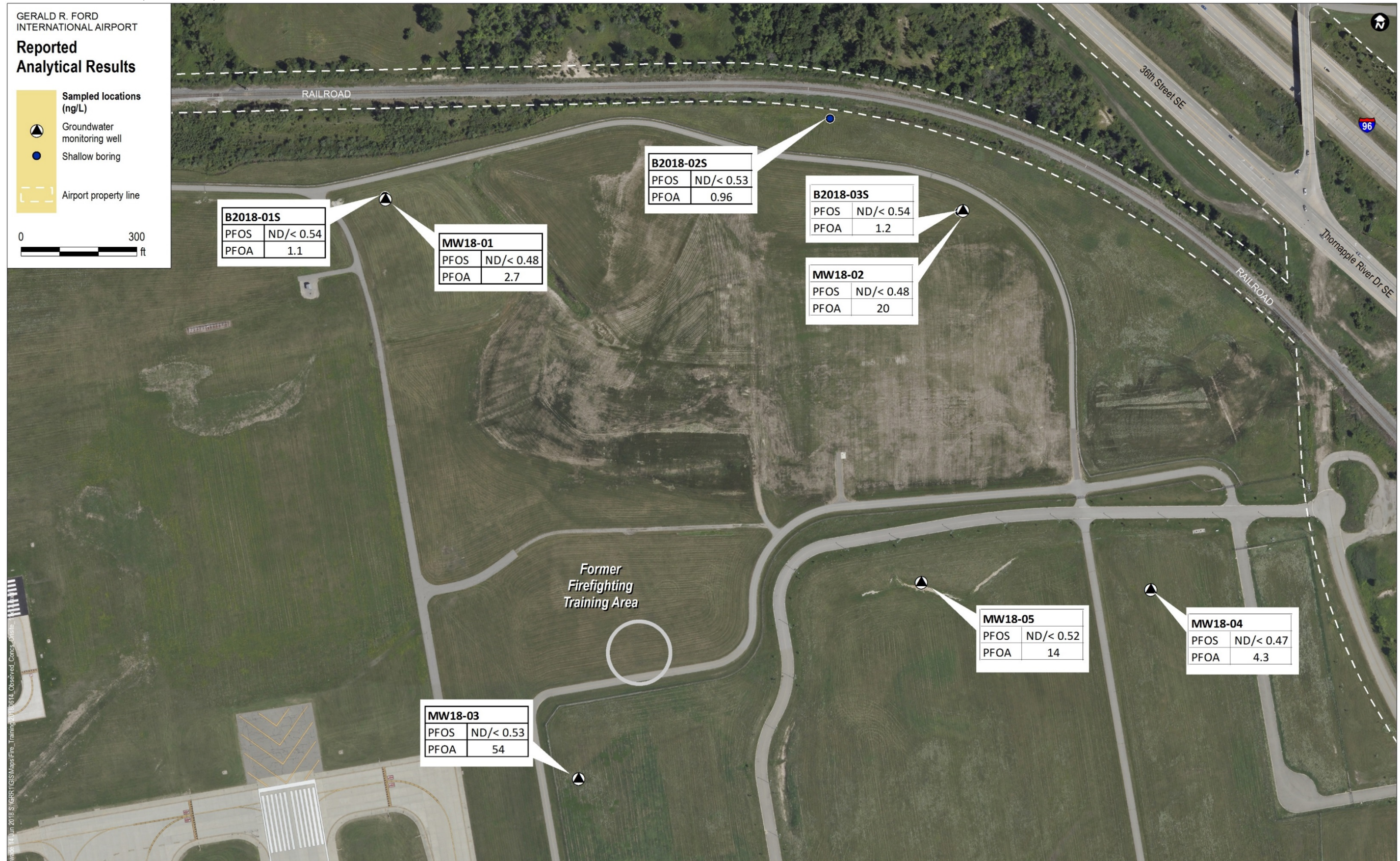
Figure 3-3. Groundwater PFOS and PFOA Sample Results (ng/L).
