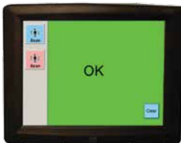
If no potential threat items are detected, an "OK" appears on the monitor with no outline.
